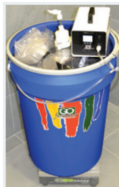
FIGURE 7 This GOfermentor JR is in the middle of pressing the wine that has finished fermentation into one of the Smart Barrel liners.
