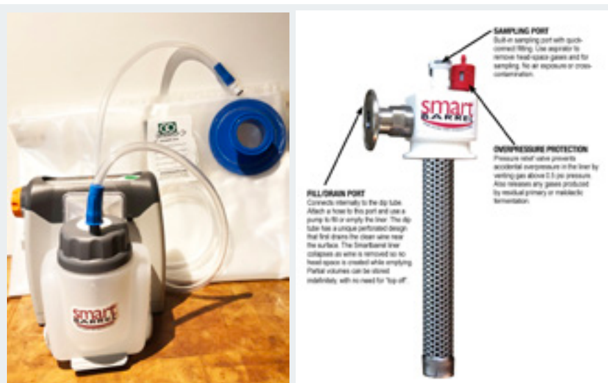
FIGURE 9 One interesting addition to GOfermentor’s equipment is their Aspirator. The flexible tube with the blue end attaches to the top of the diptube. When the aspirator is turned on, it removes any air from the GOliner and then sucks a wine sample into the bottle attached to the aspirator. This process reduces the possibility of introducing microbial contamination to the wine.
