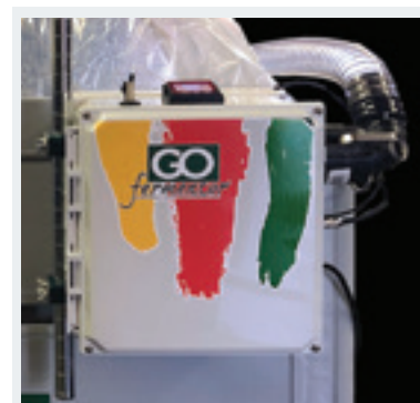
FIGURE 3 The GOfermentor controller attaches to the side of the bin and the controller screen is on top of the macrobin.
