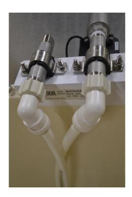
The electric valve has a cable with a DC barrel plug that must be plugged in to the jack marked VALVE located on the right side on the control panel near the power entry cable.
