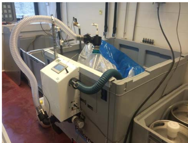
Figure 4. Tempranillo alcoholic fermentation with Gofermentor system.
